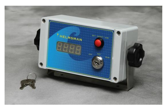
The Helmsman AW201 Watch Alarm serves two distinct functions on a marine vessel. In normal mode it operates as a watch-timer alerting the pilot periodically to ensure that full attention is maintained while at the helm. The AW201 also serves is an event counter that can keep count of pump-down cycles while the vessel is moored.
